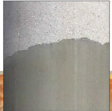
Sand column testing visually demonstrates the rapid and complete permeation achieved by US Grout Ultrafine and provides correlative data for grouting into fine, dense soils.
