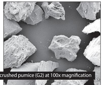
crushed pumice (G2) at 100x magnification
